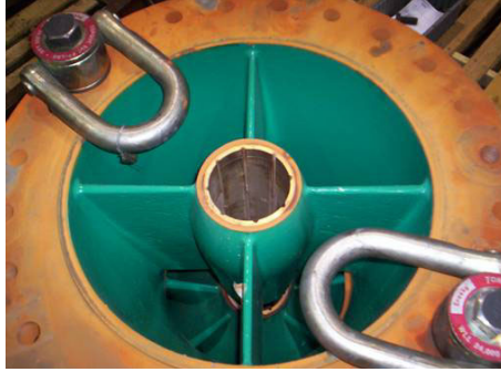
Figure 3. SK134 fusion bonded epoxy application.
