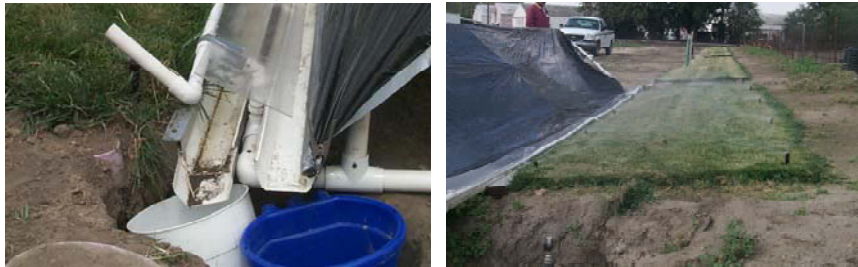
Figure 1. Left photo shows runoff collection system for surface runoff and wind drift. Right photo shows 5 by 20 foot plots and wind drift collection barrier.
