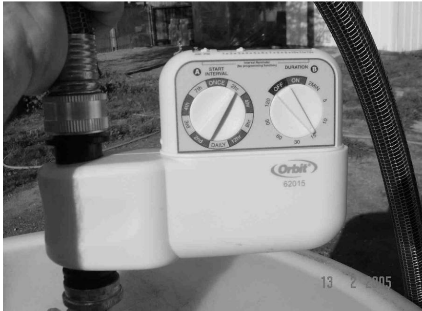
Figure 9: Spigot Mounted Inline Irrigation Water Controller, model 62015 by Orbit.
