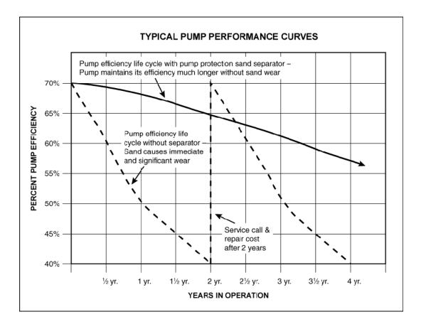
There is obvious and distinct value in protecting pumps from sand. The challenge is to apply an effective solution without the time, costs and restrictions of drilling a new well. Such solutions must take into consideration not only their relative cost, but also their suitability within the well's environment, their lifespan and, most importantly, their ability to effectively remove the sand that could damage the pump and reduce its potential longevity.
