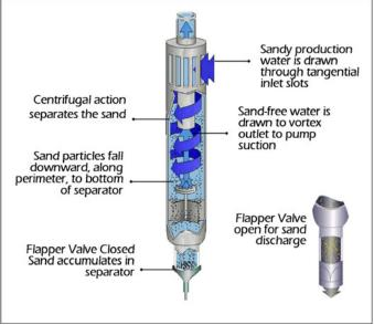
separator is fed by head pressure created by submergence. A minimum of 25-30 feet of drawdown head is required to feed proper flow through this technology. Each pump protection separator has a specific flow range that it best operates within.
