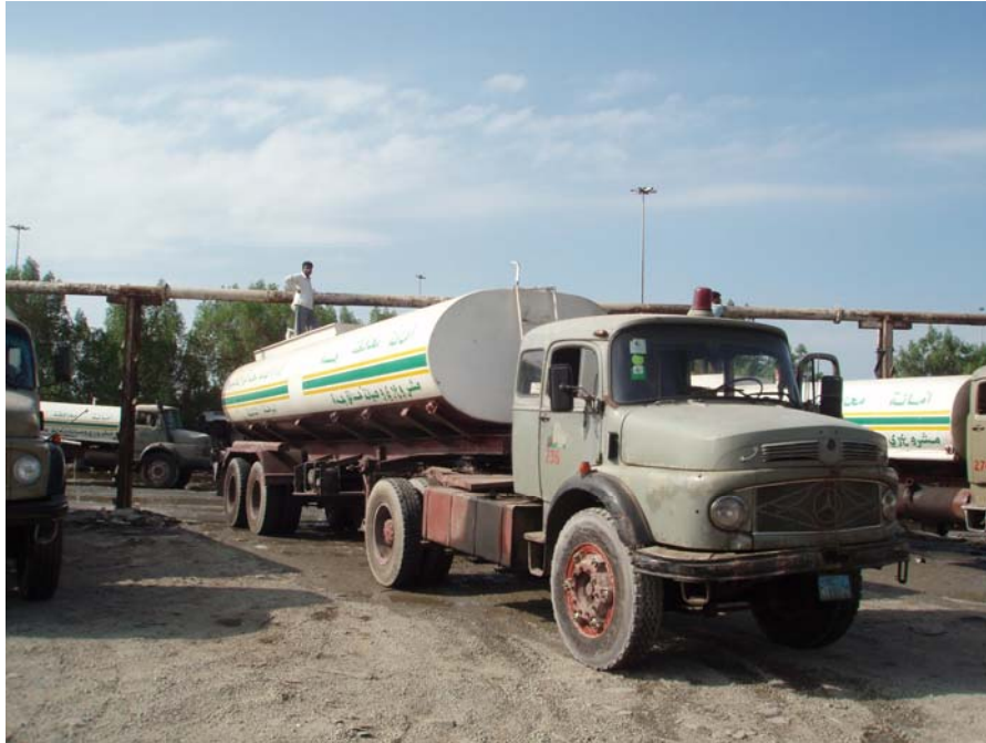
Figure 1. Tanker trucks are filled at the sewage treatment plant and recycled water is hauled to subterranean tanks throughout the community. Water is used for landscape irrigation.
