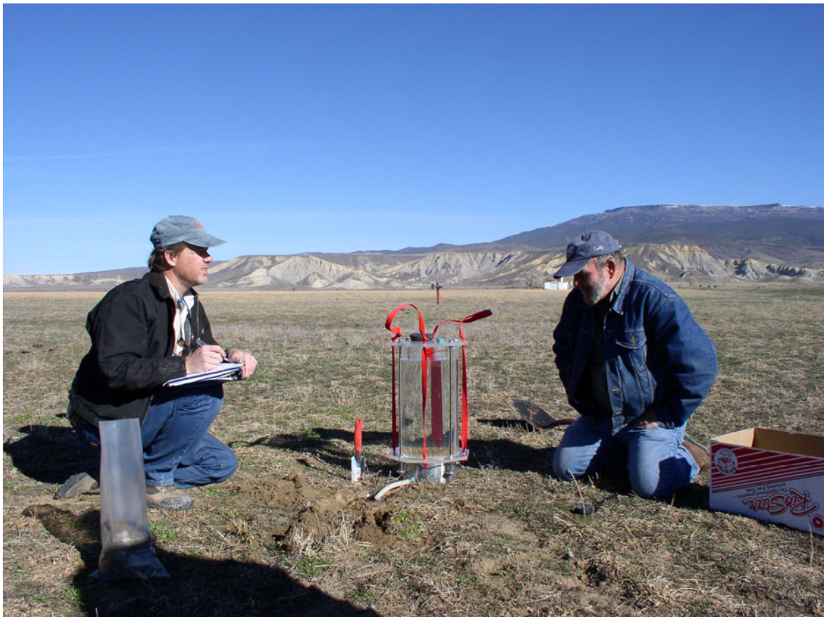
FIGURE 3: Infiltration testing with Cornell infiltrometer
