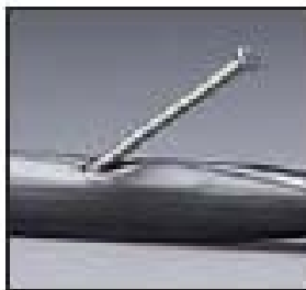
Figure 14: Holes for inserting tubing are made by inserting a nail at 45 degrees through one side of the tubing and twisting. Source: Chapin Watermatics Inc., 2007.
