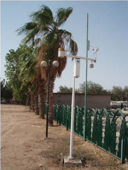
Figure 13. A portion of the landscape irrigation systems in the City of Jeddah are controlled using a central control system tied directly with a local weather station to monitor day-to-day evapotranspiration rates.
