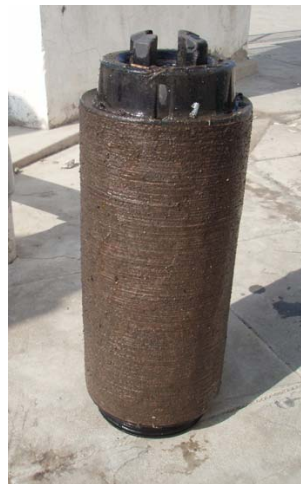
Figure 15. In the photo on the left above, the filters were disassembled to show that no filter elements were installed at the time of this site visit. In the photo on the right, the clogged filter element can be seen. This filter element was sitting off to the side -- uncleaned and unused.
