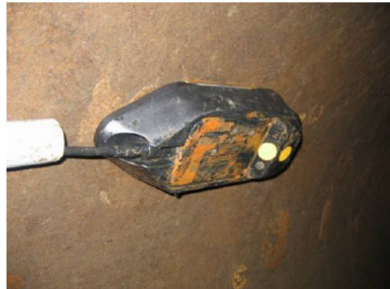
Figures 5 & 6: Photos show the installation into one of the TCCA sites. The photo at right shows the Argonaut-SW cradled in a protective "shoe" that helps deflect debris away from the instrument
