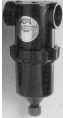
Figure 12: Aquarius Brands Incorporated 5.1 cm T-type screen filter with bottom outlet for quick flushing.
