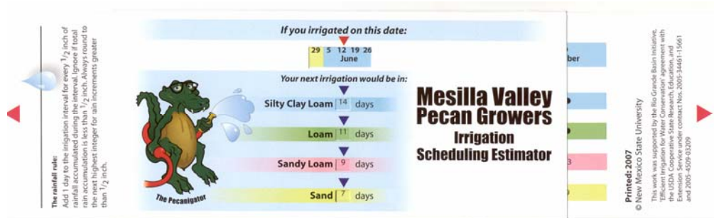
Figure 4. The printed version of the irrigation scheduling estimator tool, with the irrigation interval data for the four representative soil types arranged horizontally and listed below their corresponding calendar dates on a sliding card, and information about delaying irrigations with rainfall accumulations. The user slides the card through a printed jacket with cut out windows that align the calendar date corresponding to his last irrigation, and reads the irrigation interval from the line corresponding to his soil type.
