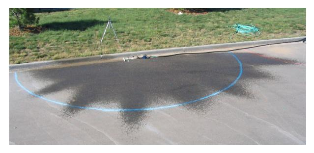
Nozzles are not manufactured equally, and most likely one batch of nozzles will not perform exactly the same as another because of molding issues. The challenge is to understand how they perform individually and then compensate for individual performance when put together in a sprinkler zone. A few of the nozzles had excellent coverage for the pattern intended, but most were not as good as would have been expected.
