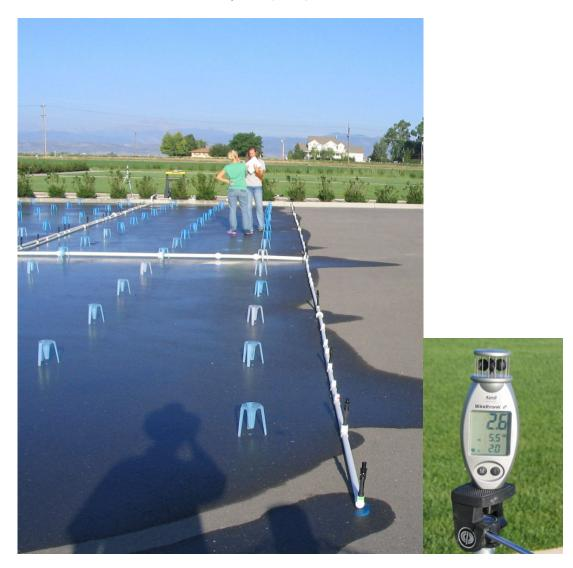
Technicians Rachel Waite and Tessa Berry gather data. A Windtronic anemometer is used to monitor wind speed during the test. It will show current speed, average wind and maximum gust during the test time. Most tests were done with an average wind speed less than three miles per hour to minimize the impact of wind on readings.
