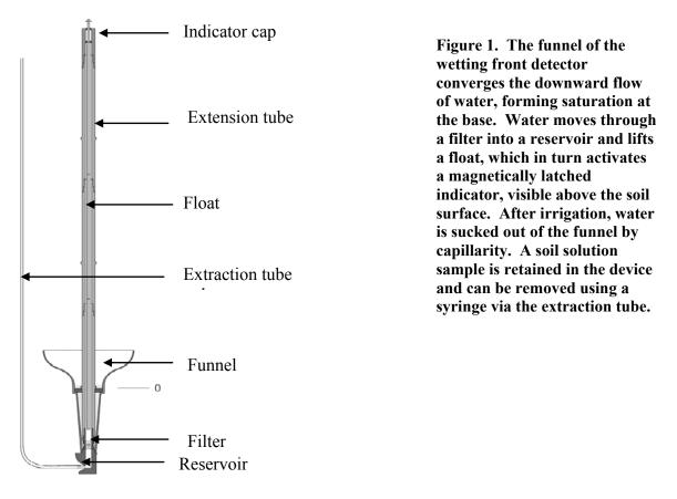
Knowing how deep a wetting front moves into the soil is critical for irrigation management. If a crop is given frequent but light sprinklings of water, the wetting front will not go deep and the WFD will not be activated. Much of the water will evaporate from the soil surface. If too much water is applied at one time, the wetting front will go deep into the soil, perhaps below the rooting depth of the crop, wasting water, nutrients and energy.
