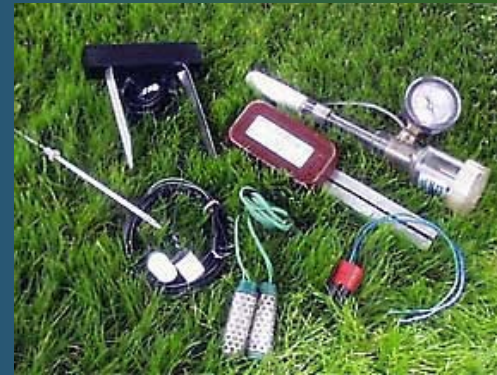
Soil Moisture Sensors
