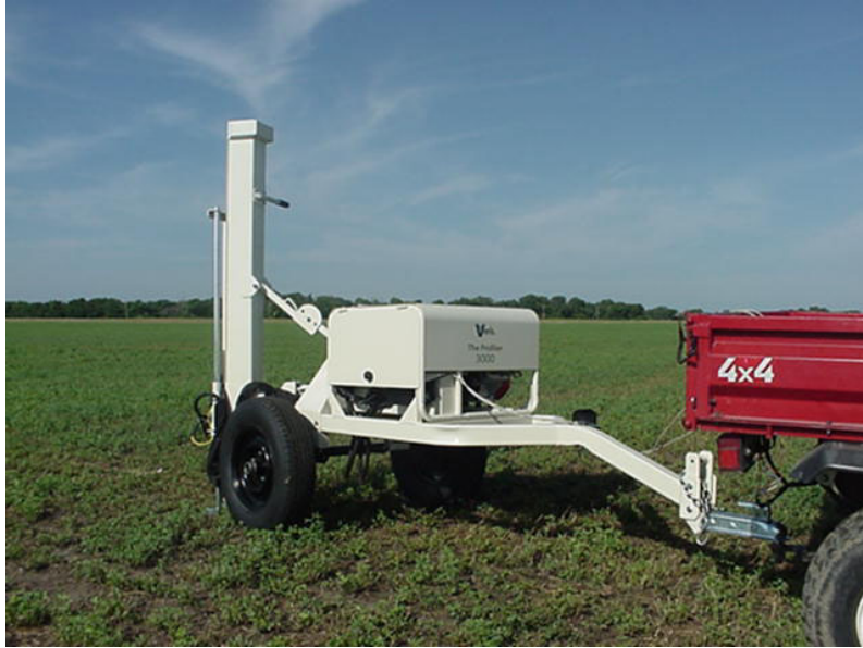
Figure 5 Soil profiler (Veris 3000) to measure soil EC and compaction.
