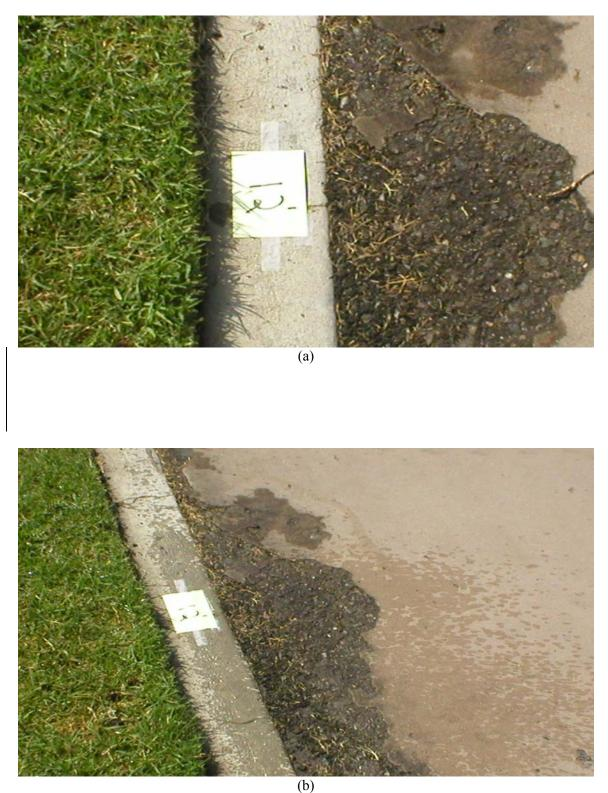
(b) **Figure 13**. Performance details of the sprinkler nozzle for the 12 ft width portion of landscape [(a) zoom view of the end point under dry conditions (b) zoom view of the end point under wet conditions]
