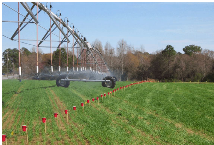
Figure 3. Catch cups underneath center pivot.
