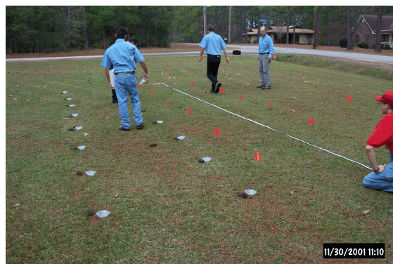
Figure 3. Installing catch-cups for a uniformity analysis at one of the audit sites.
