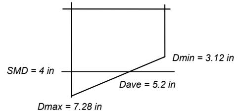
**C** 2. Given: Soil moisture depletion = 4 inches, Average infiltration = 5.2 inches, DU = 0.77.
